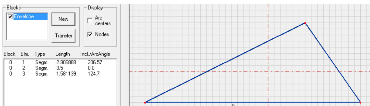
Figure B.15 – Example of situation for Error Message #2 (cf. Table 1). The envelope is composed by only 3 elements. Solution: break at least one of the line segments of the triangle.
